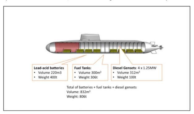
A lead-acid battery is about 13% of the displacement but only 3% of the volume of a 3,000-tonne conventional submarine. So if the 400 tonnes of lead—acid of a 3,000-tonne submarine are replaced by a light-metal battery, the volume will be the same (3% or about 220m³), but more weight must be added low in the submarine to keep its weight, stability and trim in balance.
